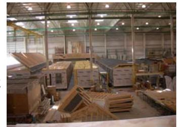
The HUD Code is the building standard to which your home is built. The HUD Code is specifically designed for compatibility with the factory production process. Performance standards for heating, plumbing, air conditioning, thermal, and electrical systems are set in the code. Also, requirements are established for structural design, construction, fire safety, energy efficiency, and transportation from the factory to the future site for the home.
